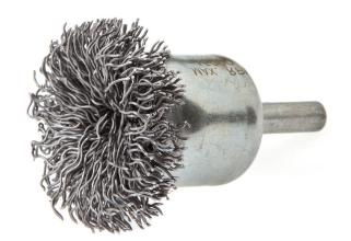
Crimped circular flared end brush. Carded. Designed for easy access into narrow holes and confined areas. For light- to medium-duty removal of rust, paint, scale, etc. Use with any 1/4" diameter electric or air tool cordless drill.
