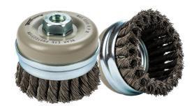
Ideal for heavy-duty cleaning of metal surfaces. Made from high carbon tempered steel. Equipped with metal bridle to eliminate flaring. When wire is worn to the metal bridle, it can be knocked off by a hammer blow exposing more wire for 30% longer life.
